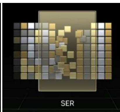
Fig. 8.2 - SER reorders threads, grouping similar work together
